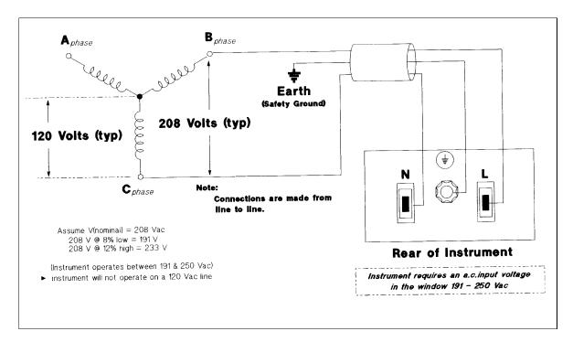
Figure 2-3. 667xA Connection to a 3-Phase Line
